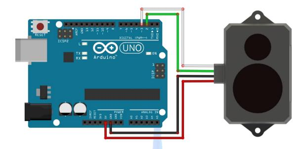
Figure 1. Wiring Diagram for TF02 and UNO Board
