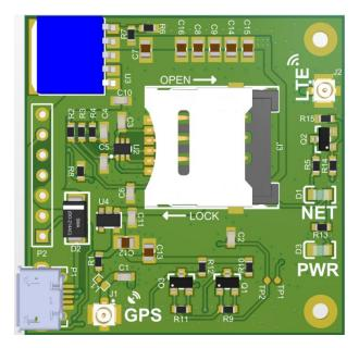
The AM76 is a system that integrates a SIM7600 series cellular module, the LTE Cat 1 module which supports wireless communication modes of LTE-TDD/LTE-FDD/HSPA+/GSM/GPRS/EDGE, it supports maximum 10Mbps downlink rate and 5Mbps uplink rate, with multiple built-in network protocols, supports drivers for main operation systems (USB driver for Windows, Linux and Android etc.) and software function.
